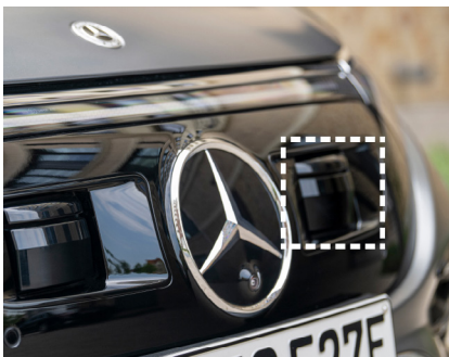
LiDAR located on front fascia
