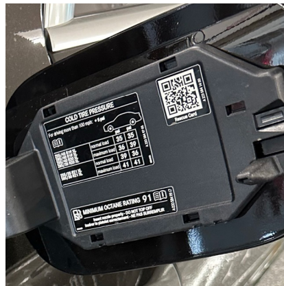
Rescue QR Code Location Fuel Filler Flap
