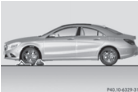
Securing the vehicle on level ground
