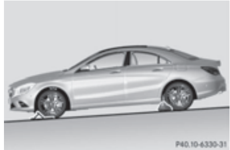
Securing the vehicle on slight downhill gradients
